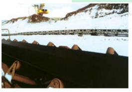
This belt can be supplied in cotton canvas, nylon canvas or EP canvas as carcass, Cover rubber is a blend of NR and BR, which has high elasticity, shock resistance, cold resistance etc, It can work @ -40°C.
