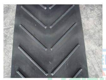
Chevron conveyor belt is suitable for conveying loose, bulky or bagged materials on inclined surface at angles of less than 40 degrees.
